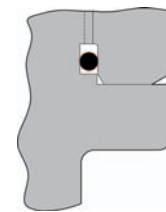
Fluoraz O-Ring Upper and Lower Body Seals in Stainless Steel Body Valves
