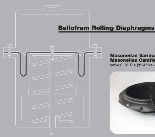
Masoneilan Varimax ATA Models 3, 5, 7 & 9 Masoneilan Camflex II Models 4 1/2" Dia (1"-2" valves), 6" Dia (3"-4" valves)
