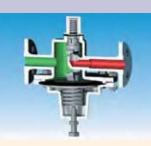
Type C3-L – Low Pressure Tank Blanketing PRV
